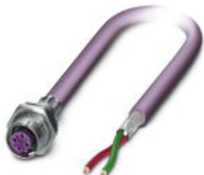
Bus system flush-type socket, PROFIBUS, 2-pos., M12, shielded, B-coded, SPEEDCON, rear/screw mounting with Pg9 thread, with 5.0 m bus cable, 2 x 0.25 mm 2
