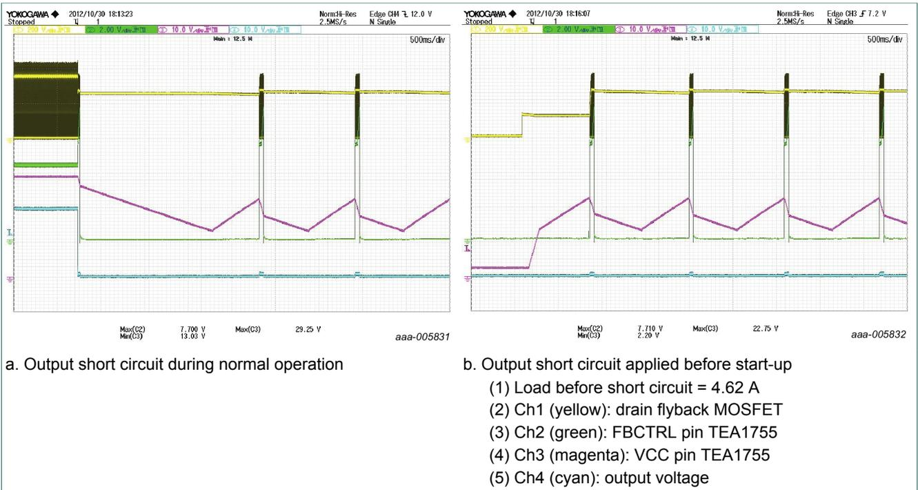
Figure 9. Output short circuit 90 V/60 Hz
