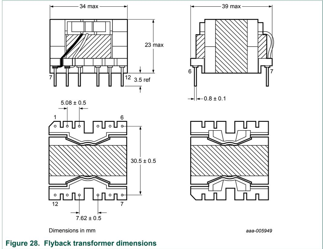
Figure 28. Flyback transformer dimensions
