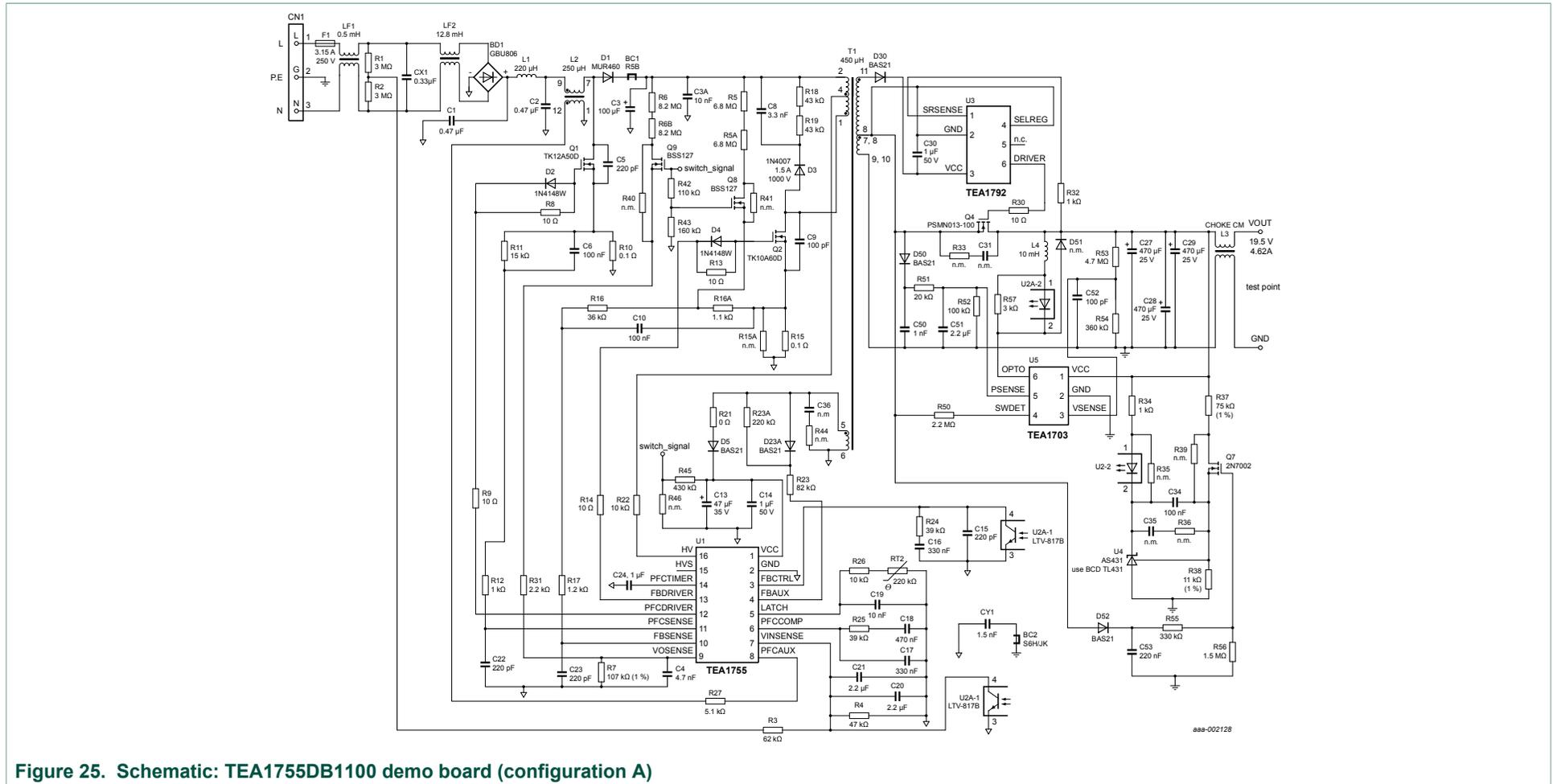
Figure 25. Schematic: TEA1755DB1100 demo board (configuration A)
