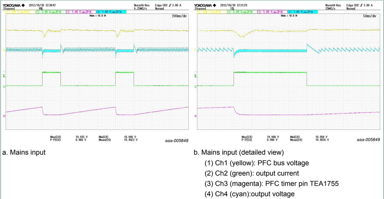
Figure 19. Dynamic load response 90 V/60 Hz
