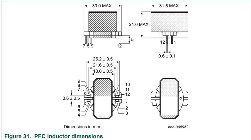
**Figure 31. PFC inductor dimensions**
