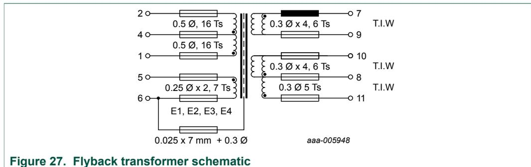
Figure 27. Flyback transformer schematic
