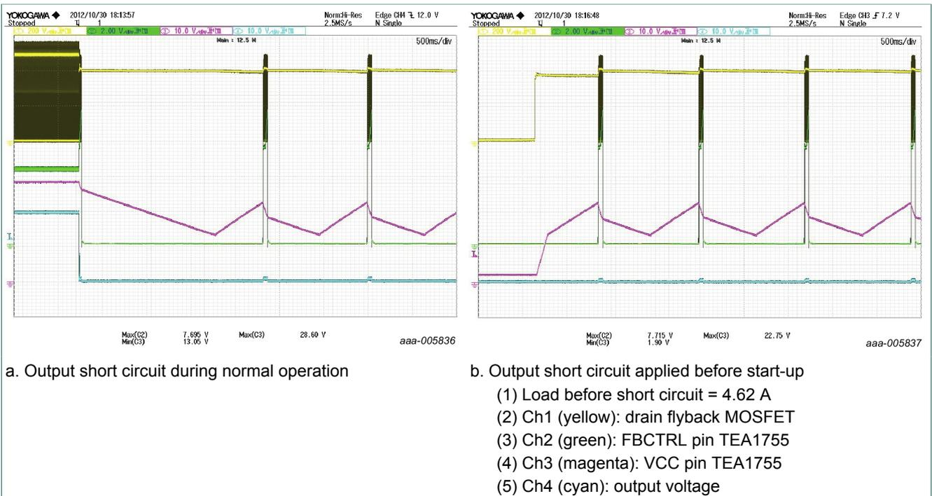
Figure 10. Output short circuit 264 V/50 Hz
