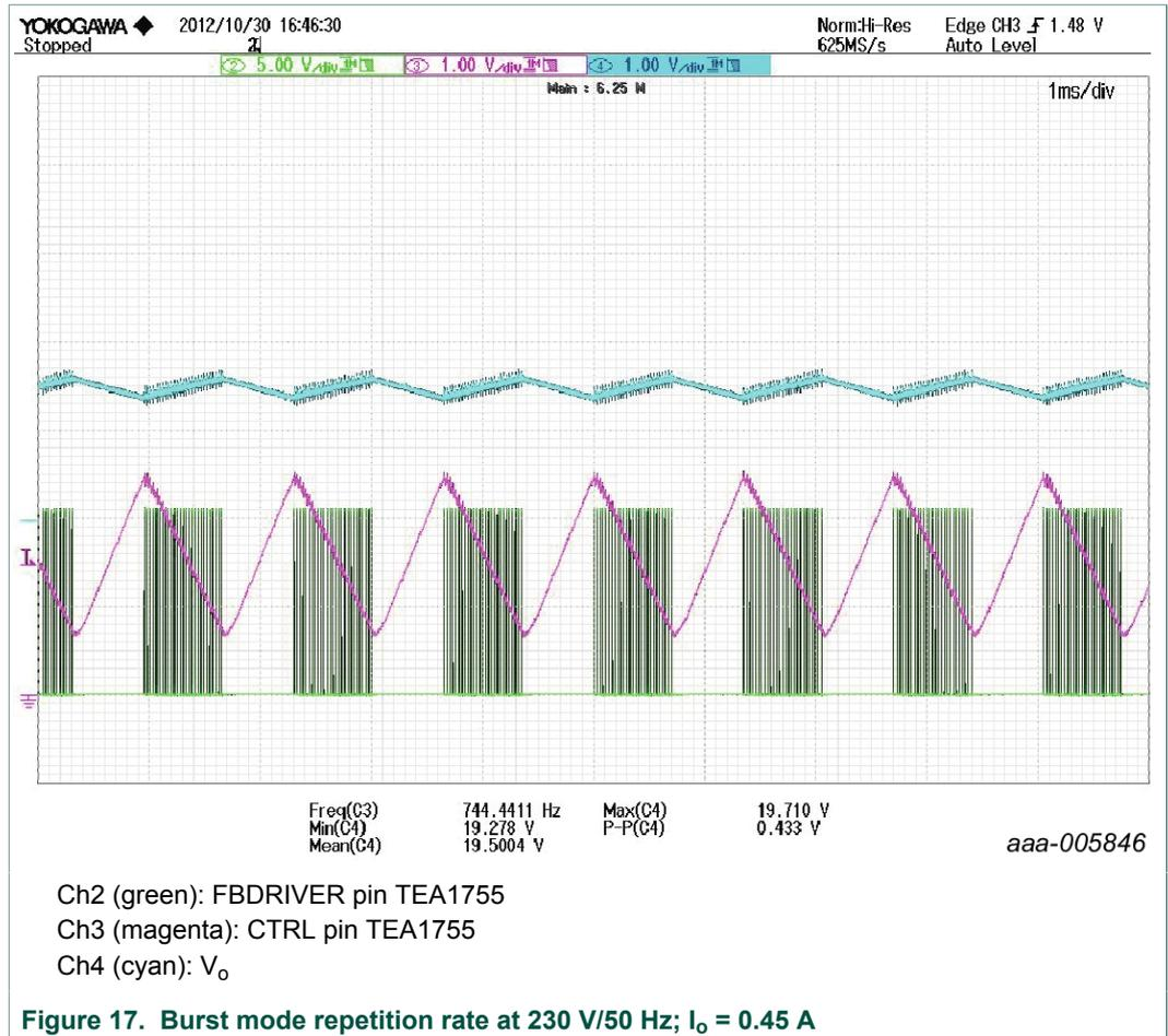
Figure 17. Burst mode repetition rate at 230 V/50 Hz;  $I_o = 0.45$  A
