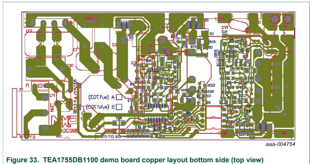
Figure 33. TEA1755DB1100 demo board copper layout bottom side (top view)
