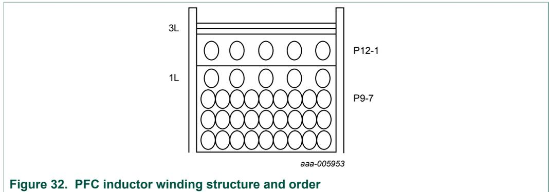
Figure 32. PFC inductor winding structure and order
