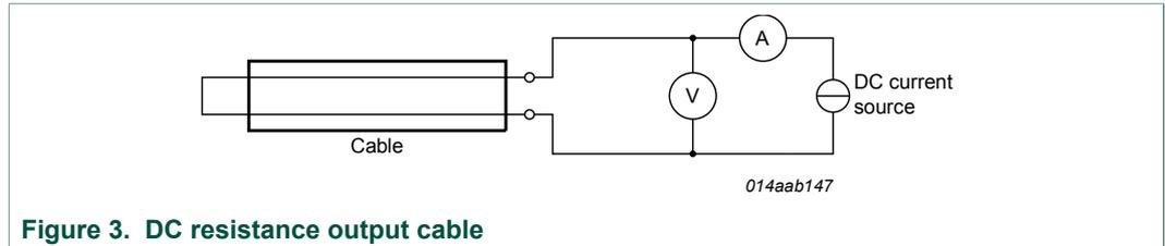
**Figure 3. DC resistance output cable**
