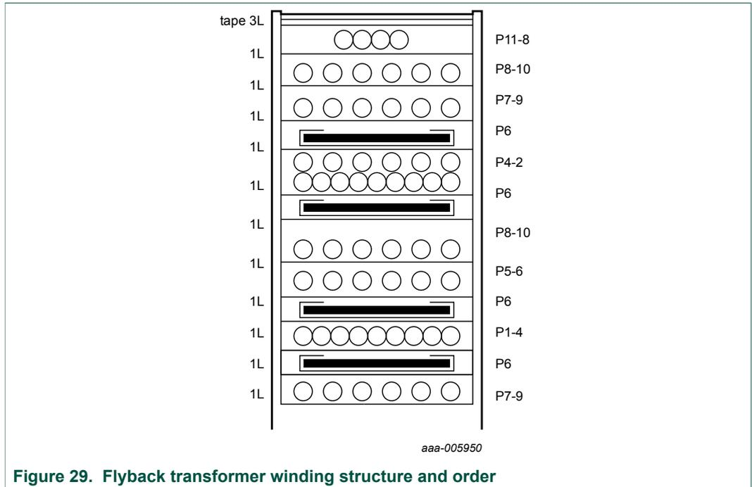
Figure 29. Flyback transformer winding structure and order
