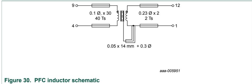
**Figure 30. PFC inductor schematic**
