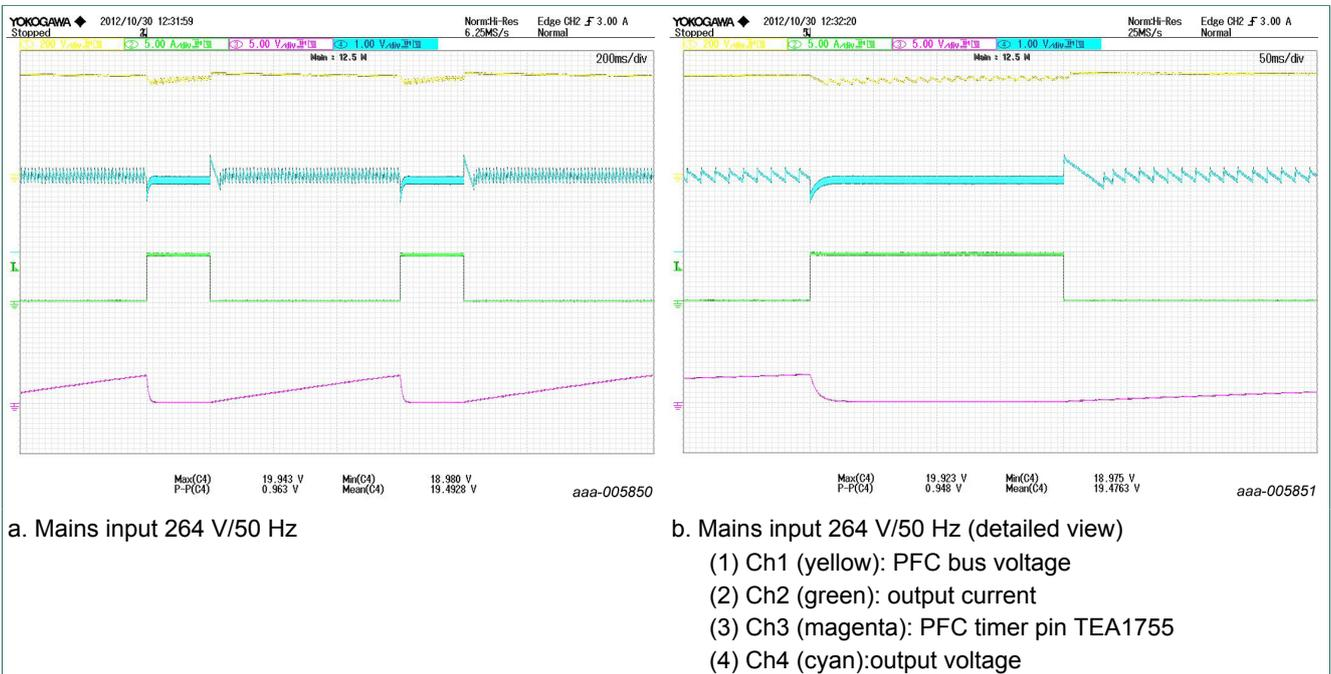
Figure 20. Dynamic load response 264 V/50 Hz
