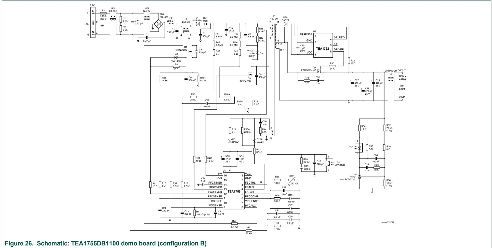
Figure 26. Schematic: TEA1755DB1100 demo board (configuration B)
