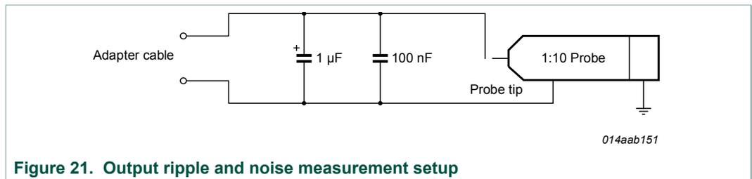
Figure 21. Output ripple and noise measurement setup
