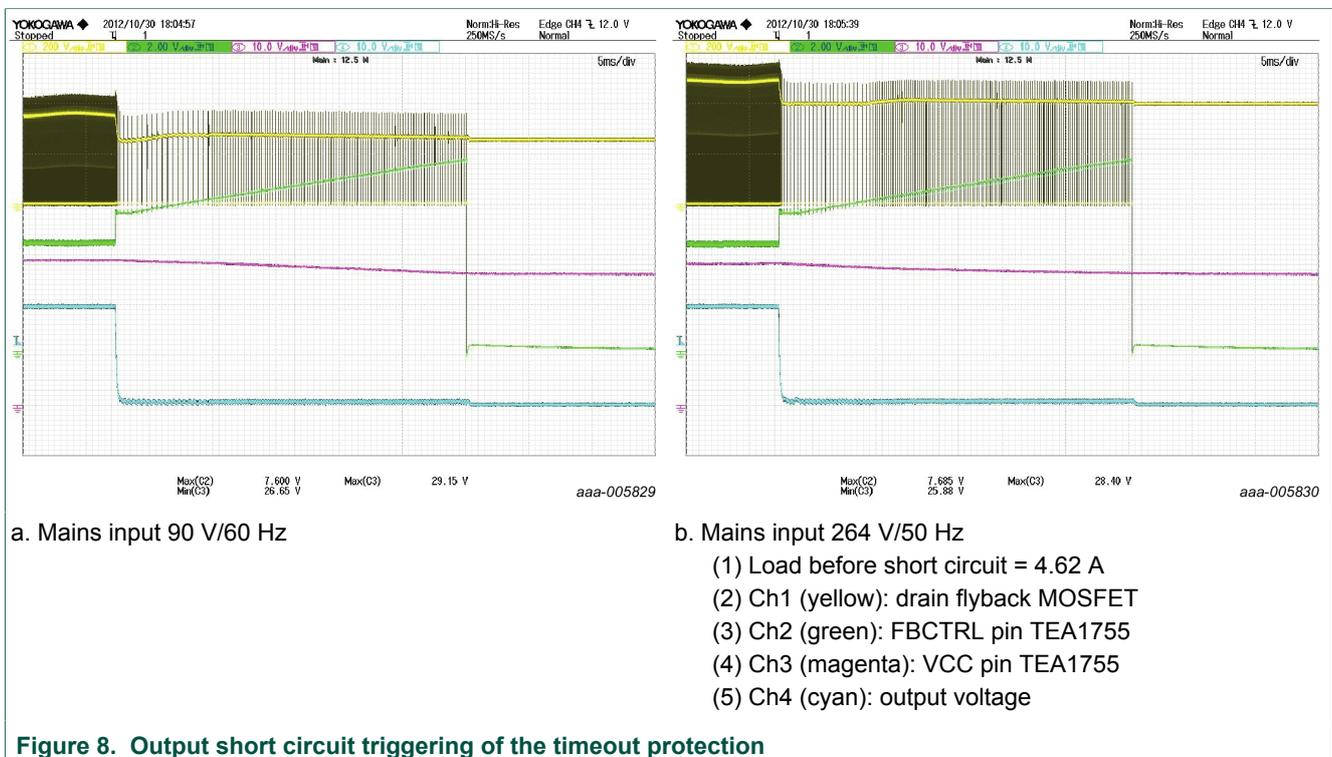
Figure 8. Output short circuit triggering of the timeout protection
