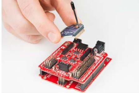
This will connect the XBee radio to the hardware serial lines of the Arduino. Next, plug your XBee Explorer into the USB port on your computer and open the serial terminal program that you were using in the *Simple Motor Control* section.
